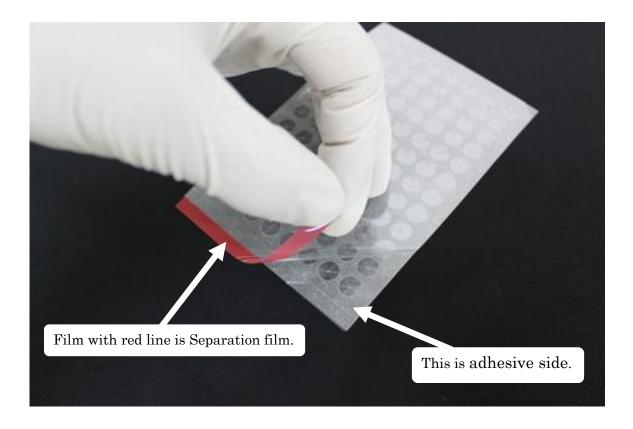
2. Seal the RAPID Slit seal to the surface of a 96-well plate correctly by adjusting well positions.
