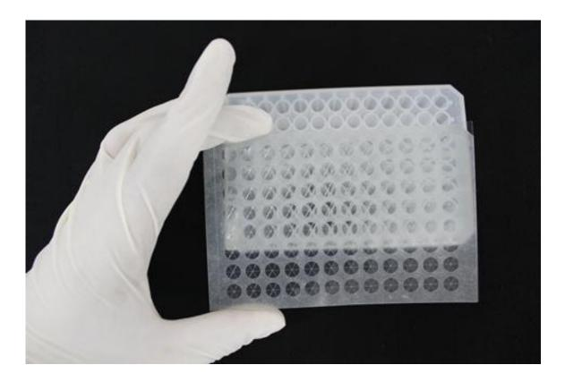
3. Remove the protection film before sampling or injection by peeling it off from the corner with precut line. Otherwise, injection needles and tips cannot penetrate into wells.
