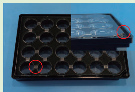
Zero-flat bottom and perfusion channel
