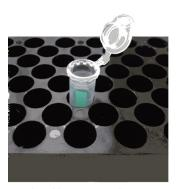
Elute by adding eluent and mixing. In case of nucleotide, approx. 90% can be eluted in 3 minutes. Paper chips can be directly put into a container, without the step to elute a sample if it is used as primer or probe.
