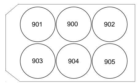
Enable efficient formation of uniformly-sized spheroids in a large quantity. Low adhesion is performed on the surface of micro-fabricated wells. EZSPHERE series have 6 types of micro-fabricated wells.
