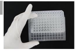
Paste the RAPID SlitSeal on the 96-well plate and make sure holes of RAPID SlitSeal are correctly positioned on each well spot.
